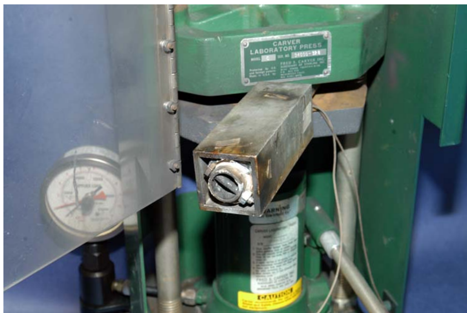
Figure 27. Photograph of heat test apparatus supported in laboratory press for testing.
