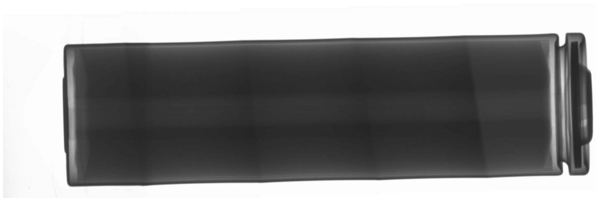
Figure 28. Exemplar commercial lithium mixed oxide cell pre-test X-ray.
