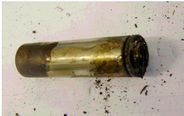
Figure 73. Photograph of a commercially available lithium mixed oxide 18650 cell after ARC testing in the closed cell configuration.
