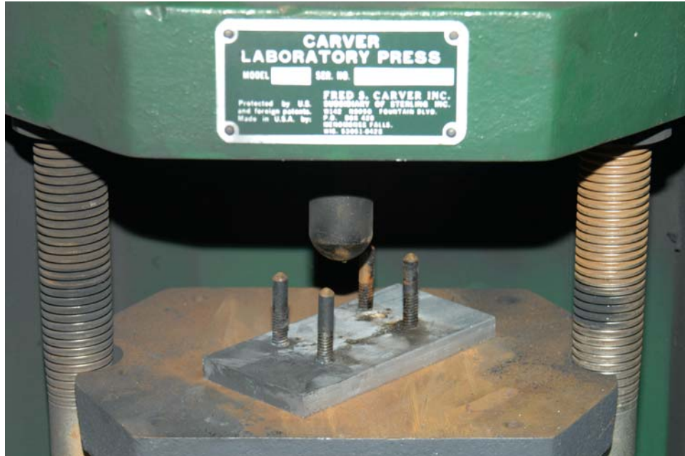
Figure 2. Photograph of crush test apparatus positioned in lab press.
