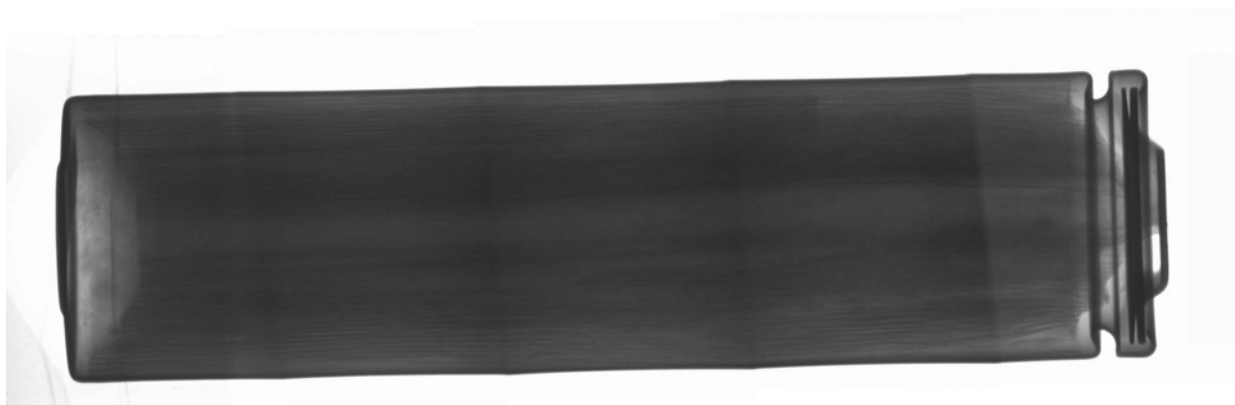
Figure 41. Post heating test X-ray image of \text{Li}(\text{Co}_{1/3}\text{Ni}_{1/3}\text{Mn}_{1/3})\text{O}_2 cell 2007149.
