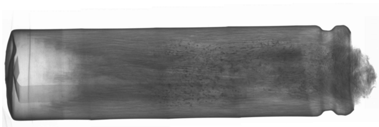
Figure 45. Post heating test X-ray image of LiCoO 2 cell 1008815.
