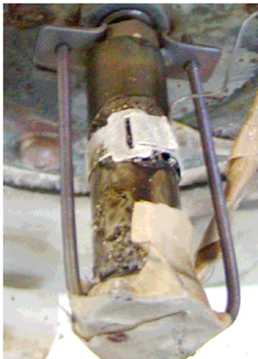
Figure 68. Photograph of Valence phosphate cell after ARC testing in the open calorimeter bomb apparatus.
