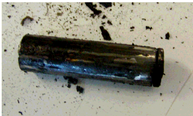
Figure 70. Photograph of a commercially available lithium mixed oxide 18650 cell after ARC testing in the open cell configuration.
