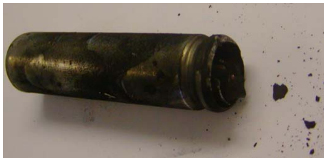
Figure 72. Photograph of a commercially available lithium cobalt oxide 18650 cell after ARC testing in the closed cell configuration.
