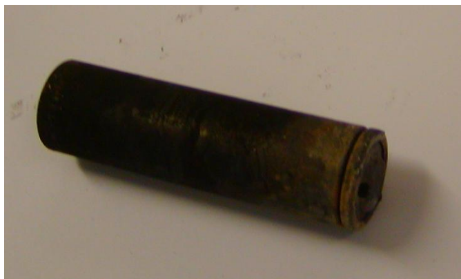
Figure 71. Photograph of Valence phosphate cell after ARC testing in the closed configuration.
