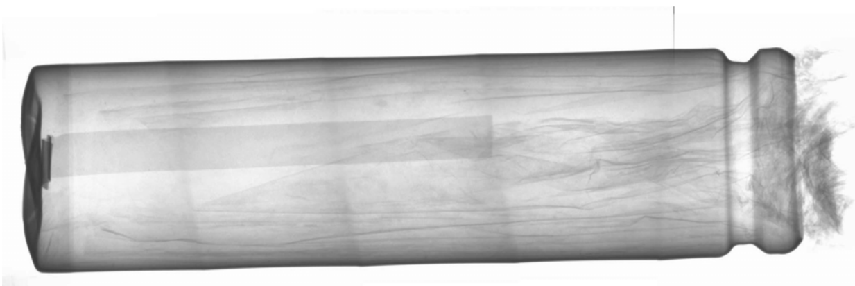
Figure 47. Post heating test X-ray image of Valence phosphate cell 15930325.
