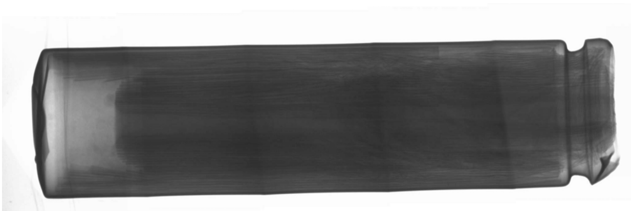
Figure 43. Post heating test X-ray image of \text{Li}(\text{Co}_{1/3}\text{Ni}_{1/3}\text{Mn}_{1/3})\text{O}_2 cell 2001015.
