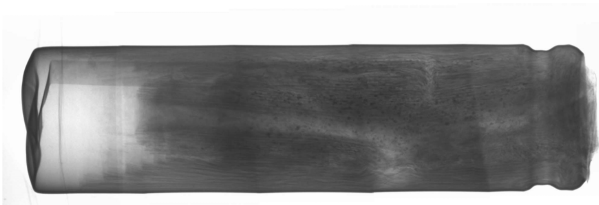
Figure 46. Post heating test X-ray image of LiCoO 2 cell 1012144.
