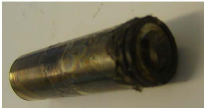
Figure 67. Photograph of Valence phosphate cell after ARC testing in the open configuration.
